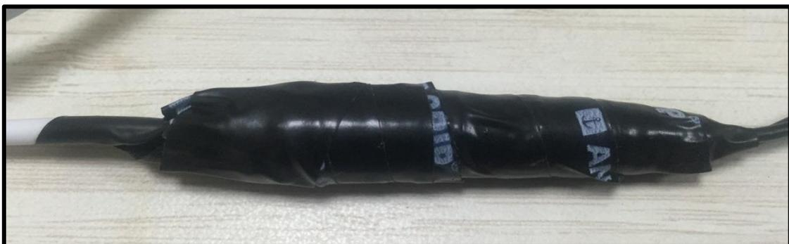
Step 4: Twist the insulation tape over the rubber tape to enhance safety.
